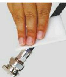
Clean the area to be applied with alcohol tissue, wipe off all the oil and dust, and wait for the alcohol to dry out;
